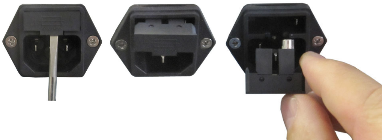
Figure 4-2. Replacing the Line Fuse
